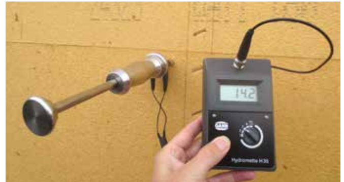
Board moisture content \leq 19.5 % with setting spruce/pine.
