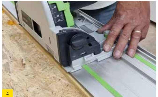
4 Saw off the sealing wedge and the two sealing corners to the required depth at the front edge.
