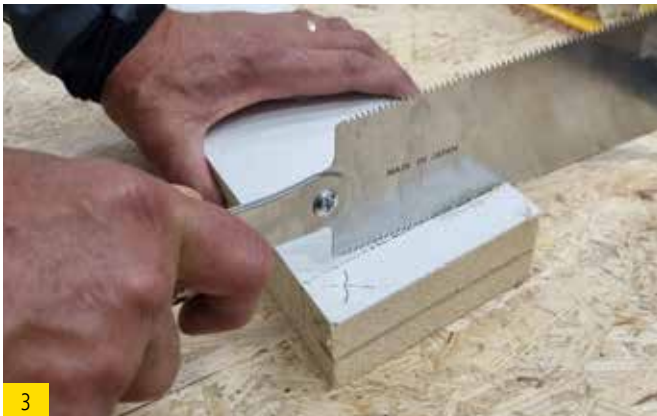
Cut out the marked area with a hand saw.
