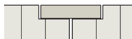
Variant 3 Standard rabbeting 23/51 mm alternatively 28/51 mm Thickness: 60–95 mm Special rabbeting up to max. 30/68 mm
